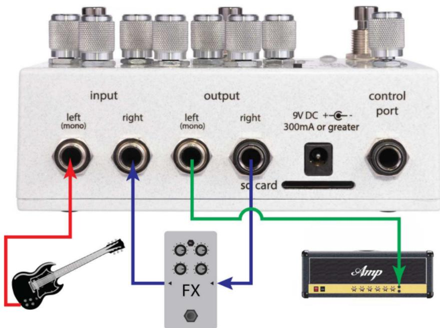
In this configuration the unit operates in mono. Left/right routing won't function as expected.
