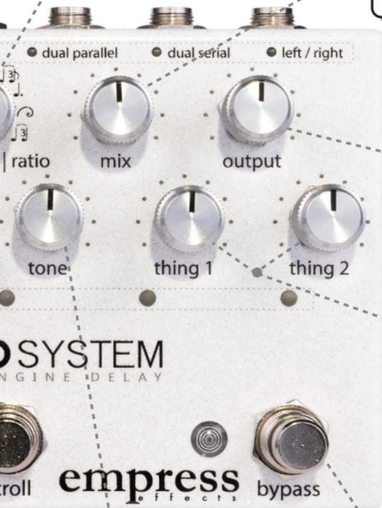
**output:** controls the overall output volume for the pedal. 12 o'clock is unity.
