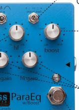
**Boost:** controls the output level. It is a clean boost, perfect for providing gain before an effects chain to minimize noise or to overdrive the input of a tube amp. The available boost ranges from 0 dB to +30 dB and is toggled on/off with the boost stompswitch.
